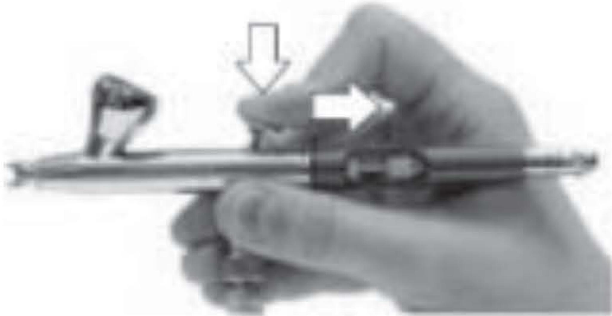
Press trigger to deliver air.
